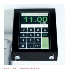
EASY - TO - USE TOUCHPAD The programmable control module is equipped with a multilingual touchpad for easy operation. 99 programs with 99 steps in each can be stored in memory.
